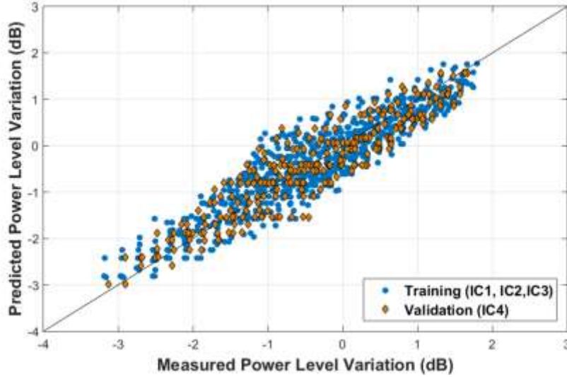
Fig. 8. Predicted power level variation vs. measured power level variation
