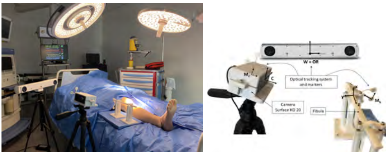
Fig. 1 Set up for optical palpation of the fibular bone using structured-light camera and localisation in the operating room using an optical tracking system
