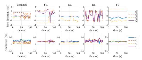
Figure 9: Time-series of the generated zero-direction angles and amplitudes for the different experimental scenarios using the SM controller.
