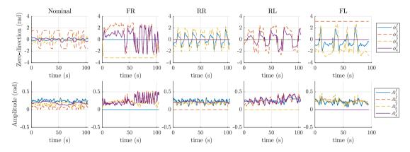
Figure 8: Time-series of the generated zero-direction angles and amplitudes for the different experimental scenarios using the PID controller.
