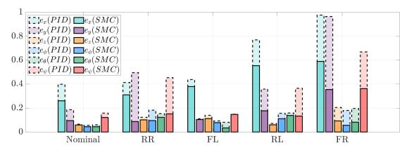
Figure 10: Bar plot of the RMS errors for trajectory tracking of all the studied scenarios. The errors for the position and orientation, expressed in meters and radians, respectively, are reported for a single trial for each case
