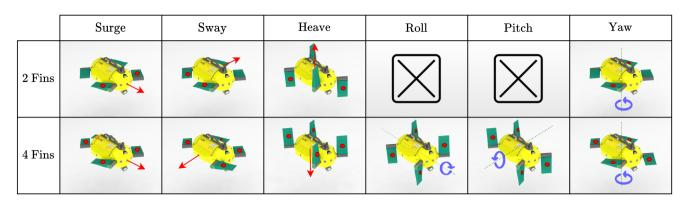
Figure 2: Illustration of the various fin configurations allowing to control the robot in each DOF using either 2 or 4 fins. The actuated fins for each configuration are highlighted with a red dot.
