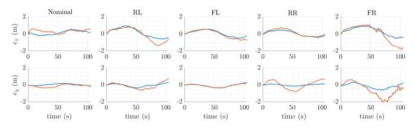
Figure 11: Tracking errors of x and y positions for all the studied scenarios. The errors are depicted for each scenario, illustrating the performance of the control strategies in various fault conditions.
