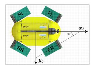
**Figure 3:** Illustration of U-CAT's fins configuration. The robot front right, rear right, rear left, and front left are denoted by FR, RR, RL, and FL, respectively.
