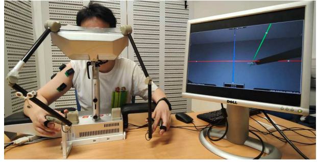
Fig. 2. 3D-printed frame in experiment (for Y-axis motion). The monitor shows the position of the Right instrument in the virtual reality.
