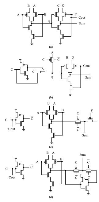
Fig. 5. The structure of the proposed approximate full adders. (a) LCAFA1, (b) LCAFA2, (c) LCAFA3, and (d) LCAFA4.
