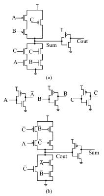
Fig. 3. The structure of the proposed approximate full adders in [17]. (a) FA1, and (b) FA2.
