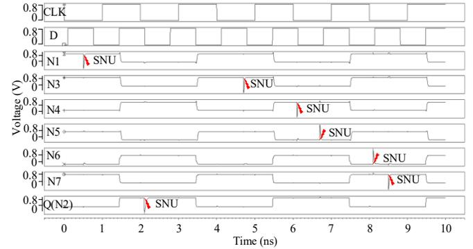
**Figure 5: Simulation results for the key SNU injections of the proposed latch.**
