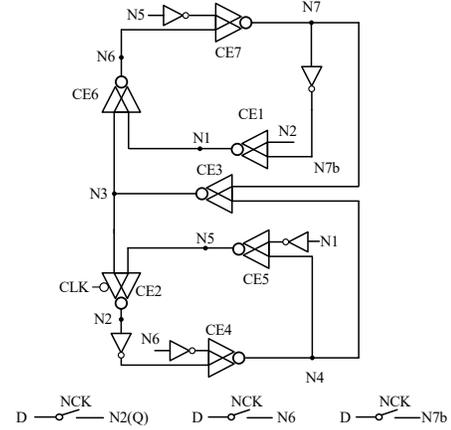
**Figure 3: Schematic of the proposed latch. Note that when CLK = 1 all transistors in TGs are ON and the latch works in transparent mode; when CLK = 0 all transistors in TGs are OFF and the latch works in hold mode.**
