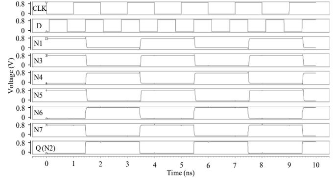
**Figure 4: Simulation result for the error-free case of operations of the proposed latch.**
