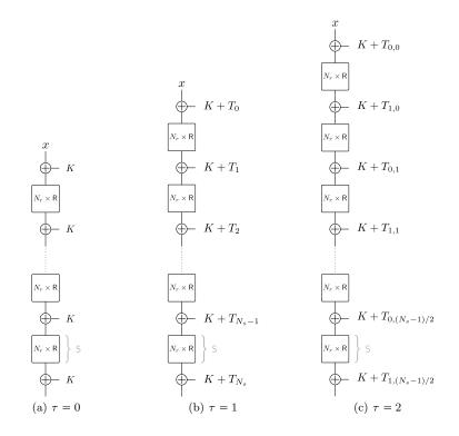
Figure 1: High-level view of FPM (tweakable) ciphers. We use the shortcut notation  $N_r \times \mathsf{R}$  to denote the application of the round  $\mathsf{R} N_r$  times.
