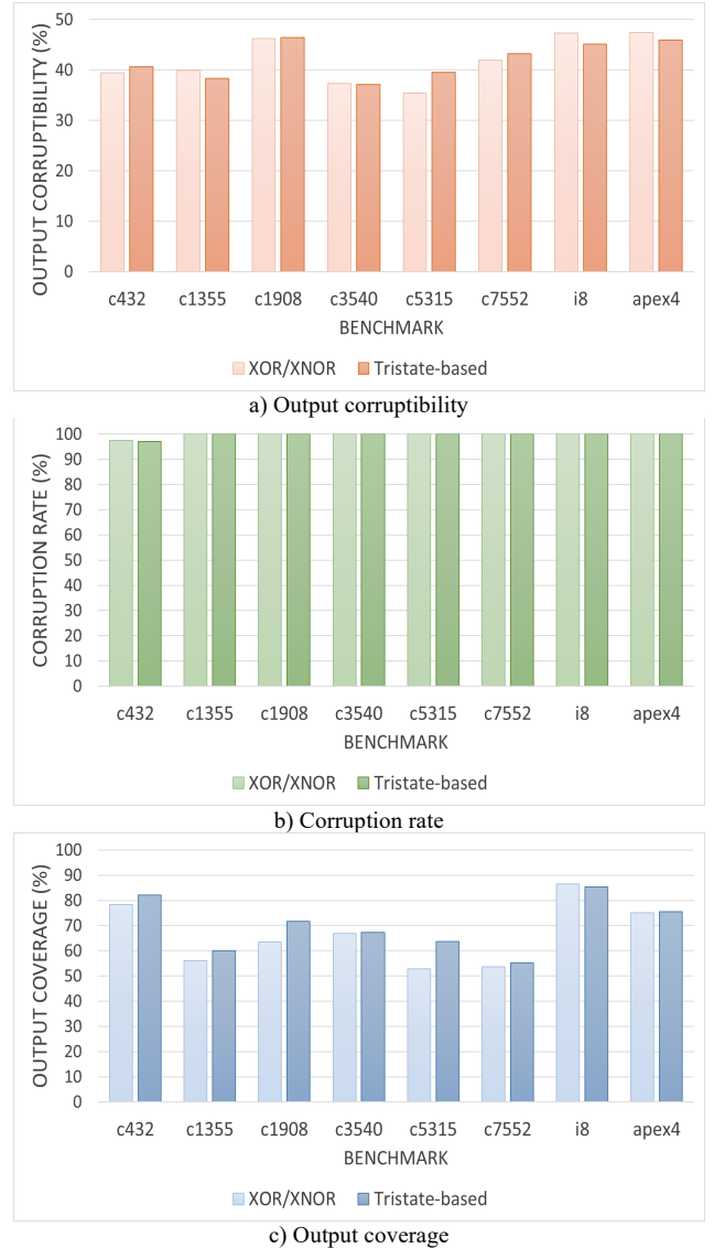
Fig. 5. Output corruption comparison, with FLL insertion algorithm
