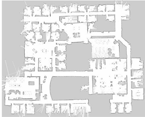
**Figure 8.** An illustrative view of the Willow environment 58.25 m x 47.25 m occupancy grid map, with 0.05 m/pixel resolution.
