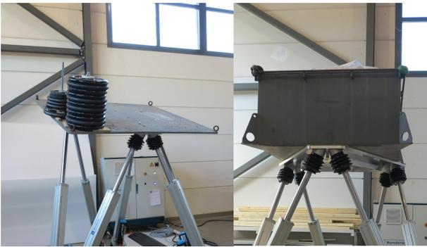
Fig. 4. Illustration of the experimental setup configurations for robustness tests, towards inertia changes (on the left), and payload changes (on the right).
