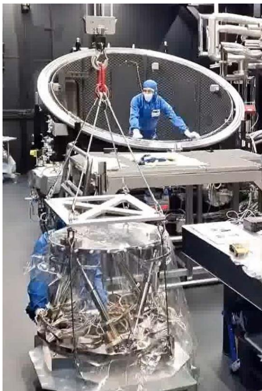
Figure 13: On the left photo of customized Zonda hexapod during installation in the thermal vacuum chamber / Copyright TNO. Stiffness compensation model principle on the right.
