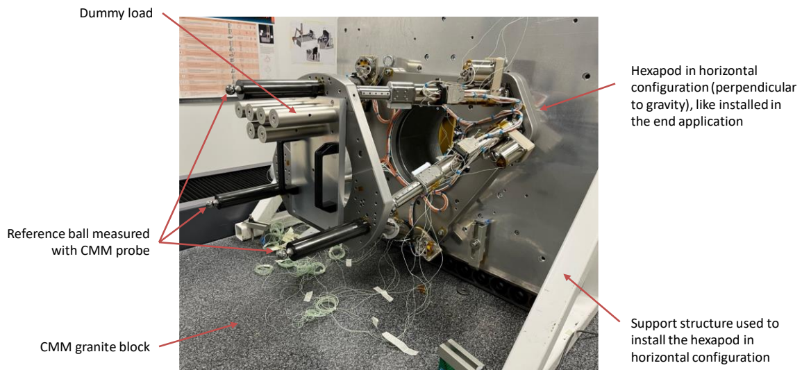
Figure 10: Setup of kinematic model calibration using a coordinate measuring machine (CMM). Here the hexapod is mounted in horizontal configuration and with a dummy load mounted on the mobile platform to be equivalent to the end application. ZONDA hexapod calibrated here is part of the SPECSID OGSE in the frame of the CHIME instrument.
