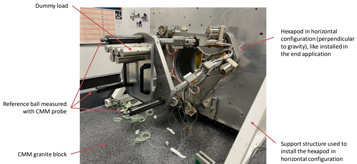
Figure 10: Setup of kinematic model calibration using a coordinate measuring machine (CMM). Here the hexapod is mounted in horizontal configuration and with a dummy load mounted on the mobile platform to be equivalent to the end application. ZONDA hexapod calibrated here is part of the SPECSID OGSE in the frame of the CHIME instrument.
