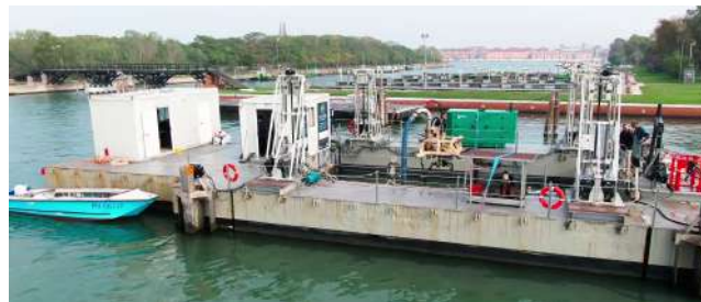
Fig. 1. The MAELSTROM project's CDP engaged in underwater litter removal: A detailed view of the mechanism, cable control from the floating barge, and litter extraction in action in the Venice's lagoon, Italy, 2022. Gouttefarde et al. (2023).
