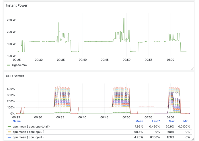
Fig. 5. Example of MCD with parallelization enabled over three consecutive runs. Each run is depicted by one of the three repeated curve patterns. The top plot shows power peaks, while the bottom plot shows CPU usage, where each colored line corresponds to one thread. It is possible to see that the parallelism appears only at the end of the algorithm.
