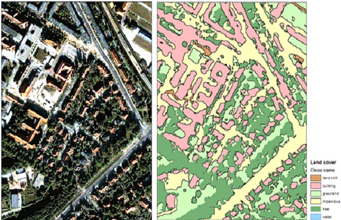
Figure 9.4: Left: Subset of a Quickbird satellite image of Rostock (© DigitalGlobe, Inc., 2011), right: derived land cover classes.
