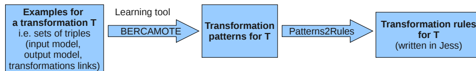
Figure 3.3 – A two-step approach for MTBE
