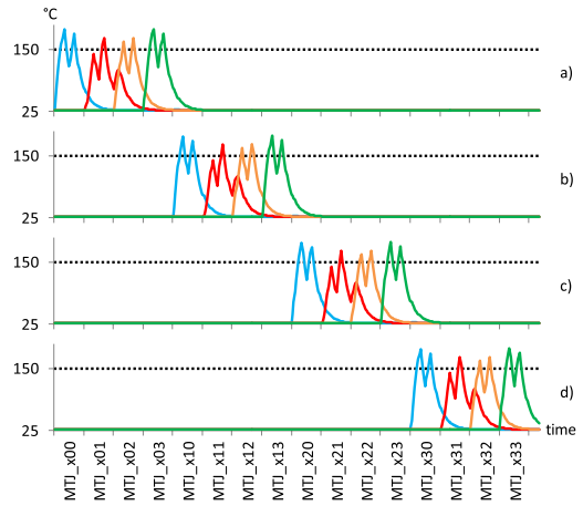
Fig. 13. 16-bit W1 temperature profile under df3 (1 M \Omega ).
