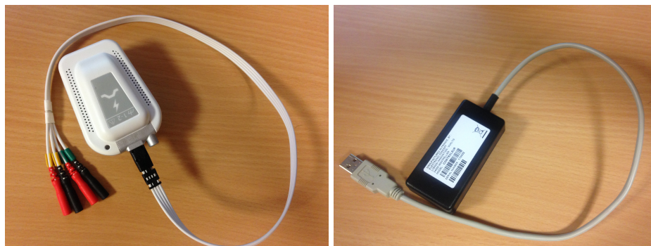
FIGURE 3.13: Wireless stimulator (Left) with its control unit (Right) (Vivaltis Inc., Montpellier, France)
