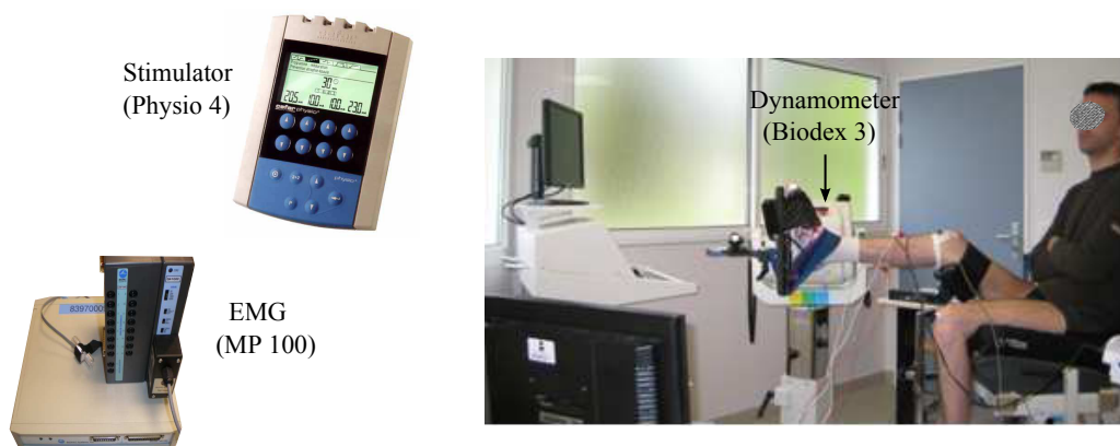
FIGURE 3.3: Experimental set-up for electrical stimulation and EMG, torque acquisition.
