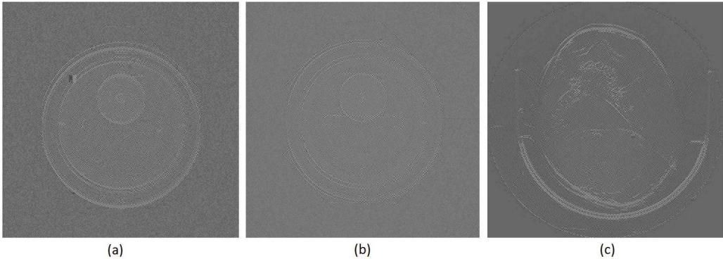
Figure 4.6: Example of the reference pattern noise from: a) the General Electric, b) The first Siemens device, c) The second Siemens device.
