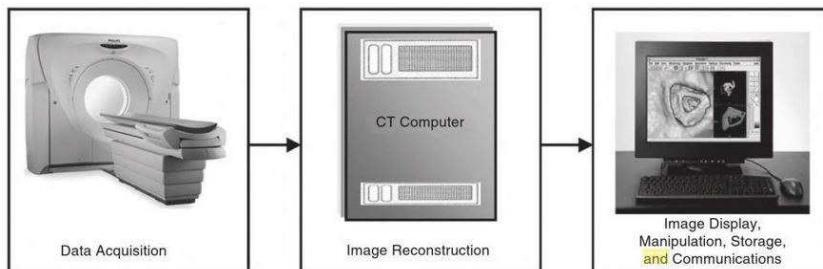
Figure 2.7: CT-Scanner imaging system [Seeram 2015]
