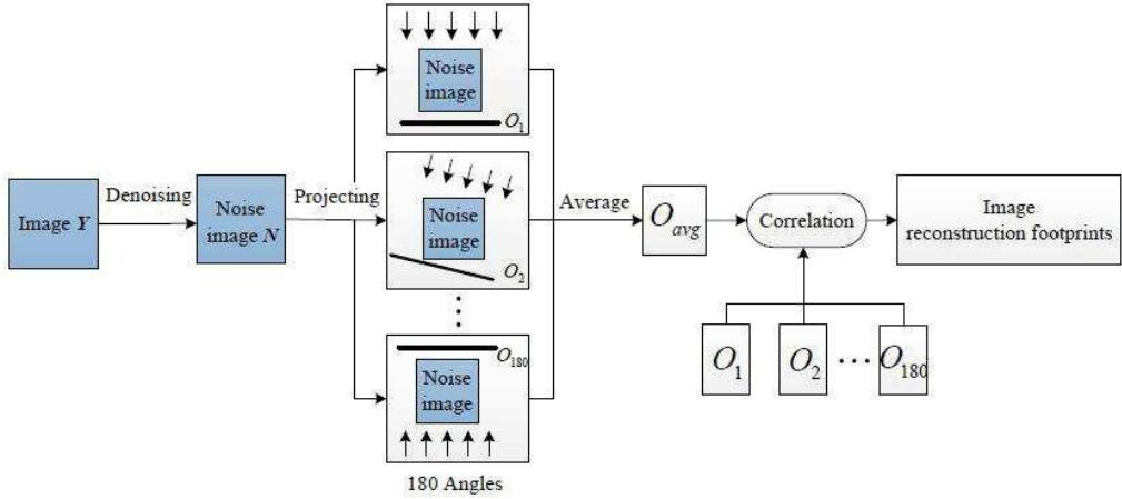
Figure 3.5: CT 3D image reconstruction algorithm footprint extraction.
