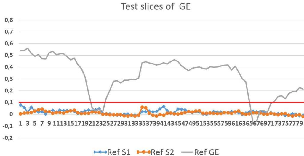
Figure 4.9: Correlations between the tested slices of General Electric and the reference noise pattern regarding each device.
