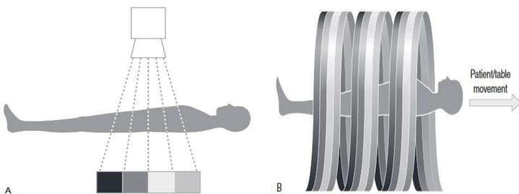
Figure 2.8: (A)Multi-detector system. (B) Multi-slice CT [Seeram 2015].
