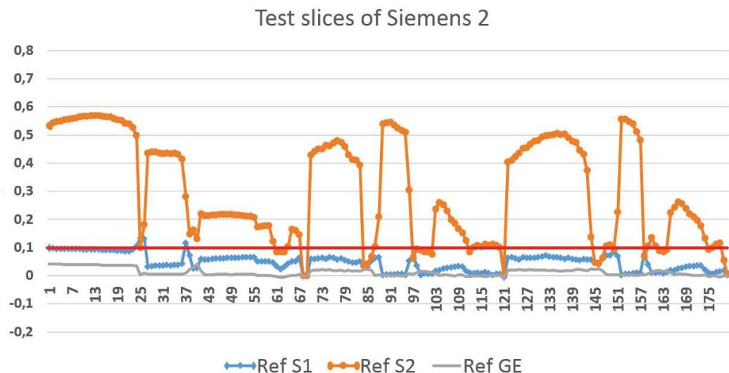
Figure 4.8: Correlations between the tested slices of Siemens 2 and the reference noise pattern regarding each device.
