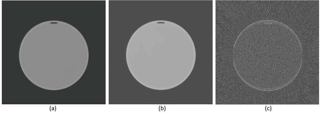
Figure 4.2: a) Example of an original slice (512x512) of a 3D image of phantom from Siemens device, b) Its denoised component, c) Its noise component.
