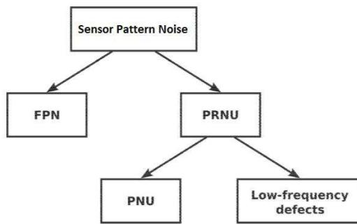
Figure 3.1: Sensor Pattern Noise
